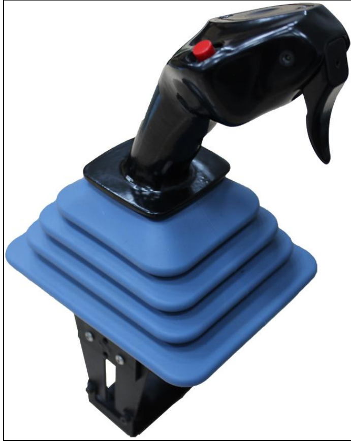
Figure 11: The Sidestick control of the A320 [10].
